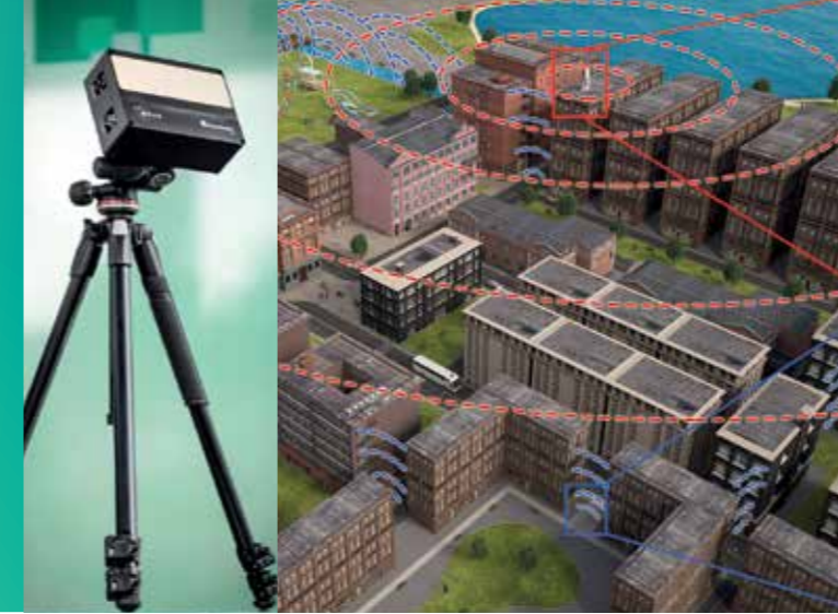
The compact and easy-to-operate radar device from Fraunhofer FHR reliably detects mini drones.
