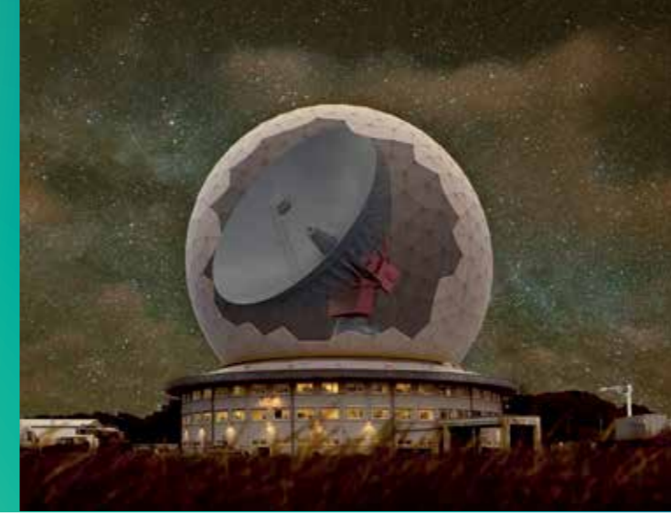
The combination of both radar systems and new complex mathematical procedures improves the accuracy of the space observation radar TIRA's distance measurement by a factor of 100.
